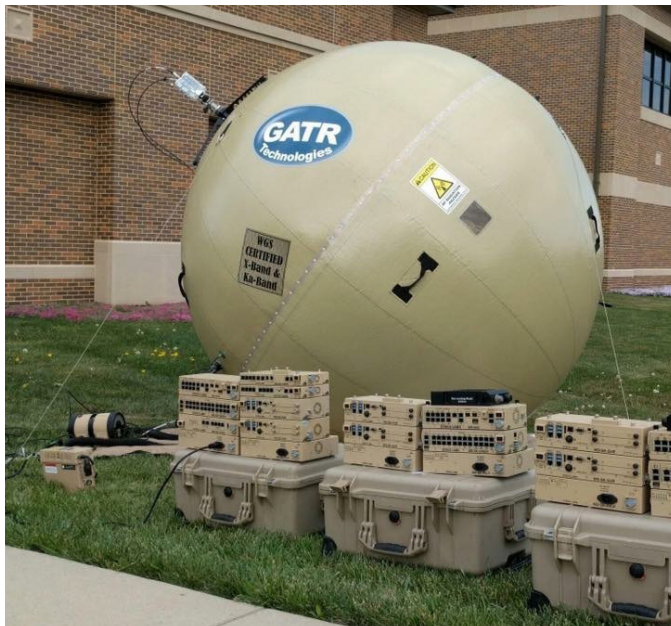
CMPS GATR inflatable satellite terminal and suite of mobile modular micro communications hardware provide customers with dramatically lower size, weight and power requirements.
