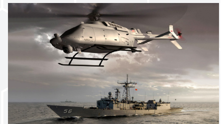
The U.S. Navy's Fire Scout MQ-8C vertical takeoff and landing unmanned air vehicle is equipped with the Dual Channel Modem for secure delivery of ISR data generated by its sensors.
