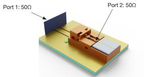
P1 is on the PCB with reference plane de-embedded to the edge of PolyStrata package. P2 is on the PolyStrata wire bonding pad. To approximate the wire bonds, an 80pH inductance is included in the plot for Return Loss and Insertion Loss (right figure).
