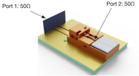
P1 is on the PCB with reference plane de-embedded to the edge of PolyStrata package. P2 is on the PolyStrata wire bonding pad. To approximate the wire bonds, an 80pH inductance is included in the plot for Return Loss and Insertion Loss (right figure).
