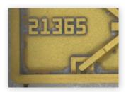
Silver may be visible in some areas on the interior of the package. This is acceptable as long as there remains complete gold coverage on the wire bond launch and the top surface of the exterior wall.
