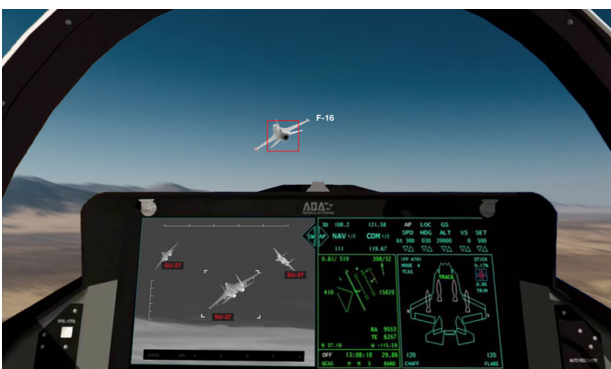
Advanced guiting capability presents aircrew with threat data across all sensor displays (RADAR, RWR, EO/IR, Others) in lieu of actual target characteristics from other LVC participants.
