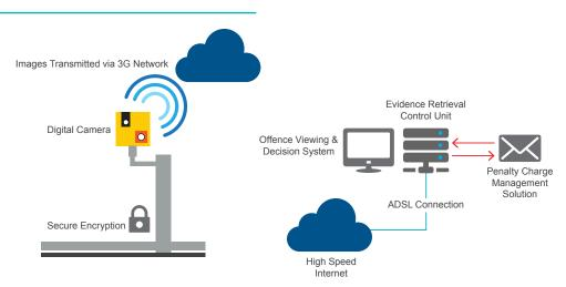
The camera can be polled by the ERCU (Evidence Retrieval Capture Unit) which is sited in the Safety Camera Partnership offices to transmit encrypted offence data via our preferred method of transmission using BT ADSL. Alternatively UTMS 3G networks can be used subject to network availability. Encrypted offence data can then be transferred to DVD disc and decrypted by the OVDS (Offence Viewing & Decision System) computer prior to adjudication through the EROS 2 or the StarTraq BOF.
